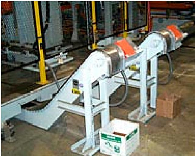
stampings, turnings, chips, fasteners and scrap. The liquid tight sealed conveyor housing can be completely submerged in machine reservoir tanks and the internal self-adjusting take up system eliminates the need for maintenance. MPI conveyors are offered with many design options and can also be supplied with other ancillary components such as feeders, hoppers, etc. to provide a complete
