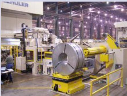
All functions are motorized and positioned by the Job Recipe to simplify and speed set-up. Ten fully-networked servo axis' are provided within the system.
