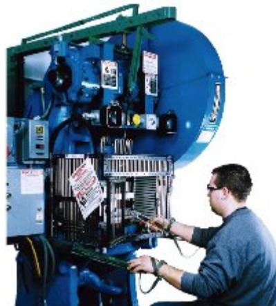
In reality a full revolution clutch may be appropriate for a simple automatic job; however, they are generally not effective for hand fed operations. Before an employer spends the necessary funds to make the full revolution clutch press comply alternate higher productivity solutions should be considered:
