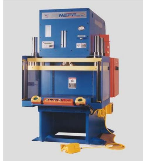
**Air over oil hydraulic presses.** These “cylinders” can be purchased configured as a press with a two hand control. If the job involves piercing, joining, coining, etc. and the load is fairly balanced these presses are an attractive affordable alternative. Tonnages are available up to 70 tons rated over ½” while total stroke is usually 6”.
