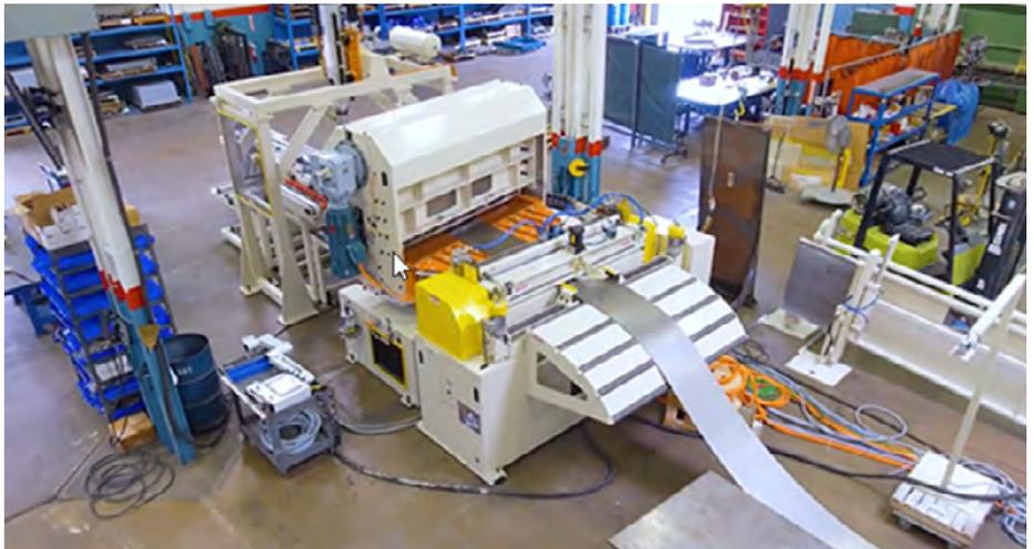
Other design enhancements include high-strength construction frame materials, tighter straightener roll spacing, and increased roll depth penetration. The new straightener heads also are equipped with increased roll
