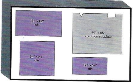
The three rectangular die sizes illustrated all can be accommodated on a common subplate measuring 60 in. by 65 in. Subplates are notched for easy location on the press bed.
