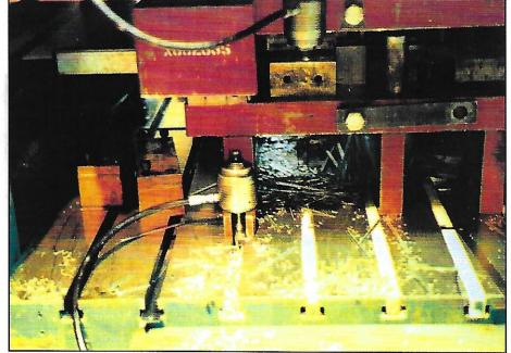
Locating a large progressive die takes a considerable amount of time when scrap must first be removed. Use of a subplate can help to minimize this problem since most scrap will be retained on the plate and removed with the old die.
