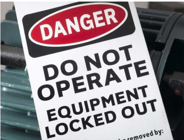
Whenever a conveyor is under repair or maintenance, it must be stopped with power sources locked out and tagged out. Exceptions may be given to conveyors that need power for testing or making minor adjustments. For more about “alternative LOTO measures” consult ANSI/ASSE Z244.1 for expanded
