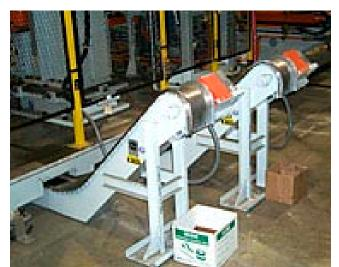
stampings, turnings, chips, fasteners and scrap. The liquid tight sealed conveyor housing can be completely submerged in machine reservoir tanks and the internal self-adjusting take up system eliminates the need for maintenance. MPI conveyors are offered with many design options and can also be supplied with other ancillary components such as feeders, hoppers, etc. to provide a complete
