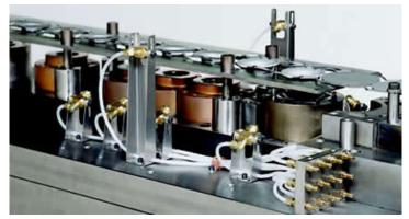
Attached Spray Nozzles & Bracket
