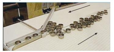
With the correct guiding, speed and belting, conveyors solve these bottlenecking issues. Dorner provides accumulation solutions using a recirculation method, allowing the product to keep moving in a stirring motion before the transfer.
