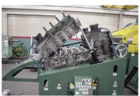
and stainless steels with critical finish requirements. The rolls can be easily inspected to ensure they are clean and free of debris that might mark the material surface.
