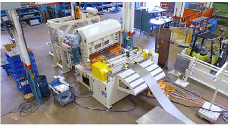
force delivery, stronger gears and bearings, and an improved straightener roller backup mechanism to provide the rigidity needed to process AHSS materials effectively. This technology has produced repeatable blanks with flatness of +/- .00035 over 18 square inches.
