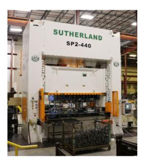
**SP2-440 TON** 10" Stroke, 24" Die Height 10" Slide Adjustment, 20-40 SPM, 120" x 60" Bolster Area I-PRESS AB PLUS CONTROL
