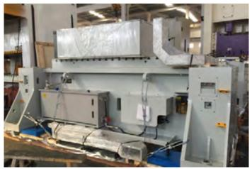
You are viewing the rear side of the bed / base which house our automatic lubrication system, tank, pumps and filters. Multiple piece tie rod construction are easy to align and assemble with our round tapered stack up alignment keys.
