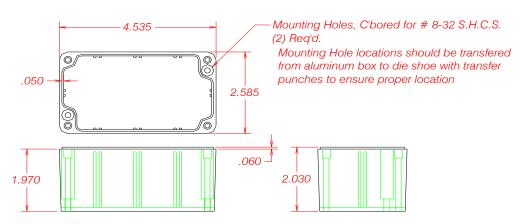
Cast Aluminum Box for HD19 Kit Comes complete with fasteners to secure Cover plate to box, and urethane rope gasket to seal cover plate water/oil tight
