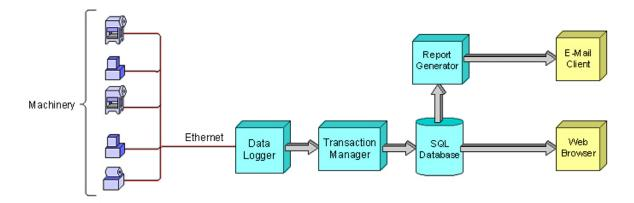
Figure 1 - Block Diagram of a Data Collection System
